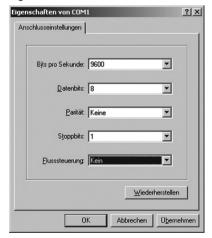
Fig. 25 Definition of the serial interface
